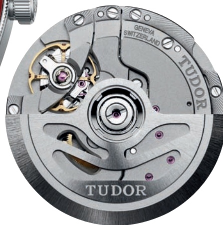
The Manufacture Calibre MT5652 powers the Black Bay GMT
