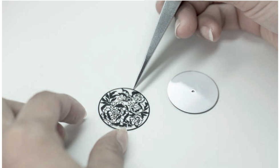
The paper motif is applied with glue on the base of the dial made of Grand Feu enamel
